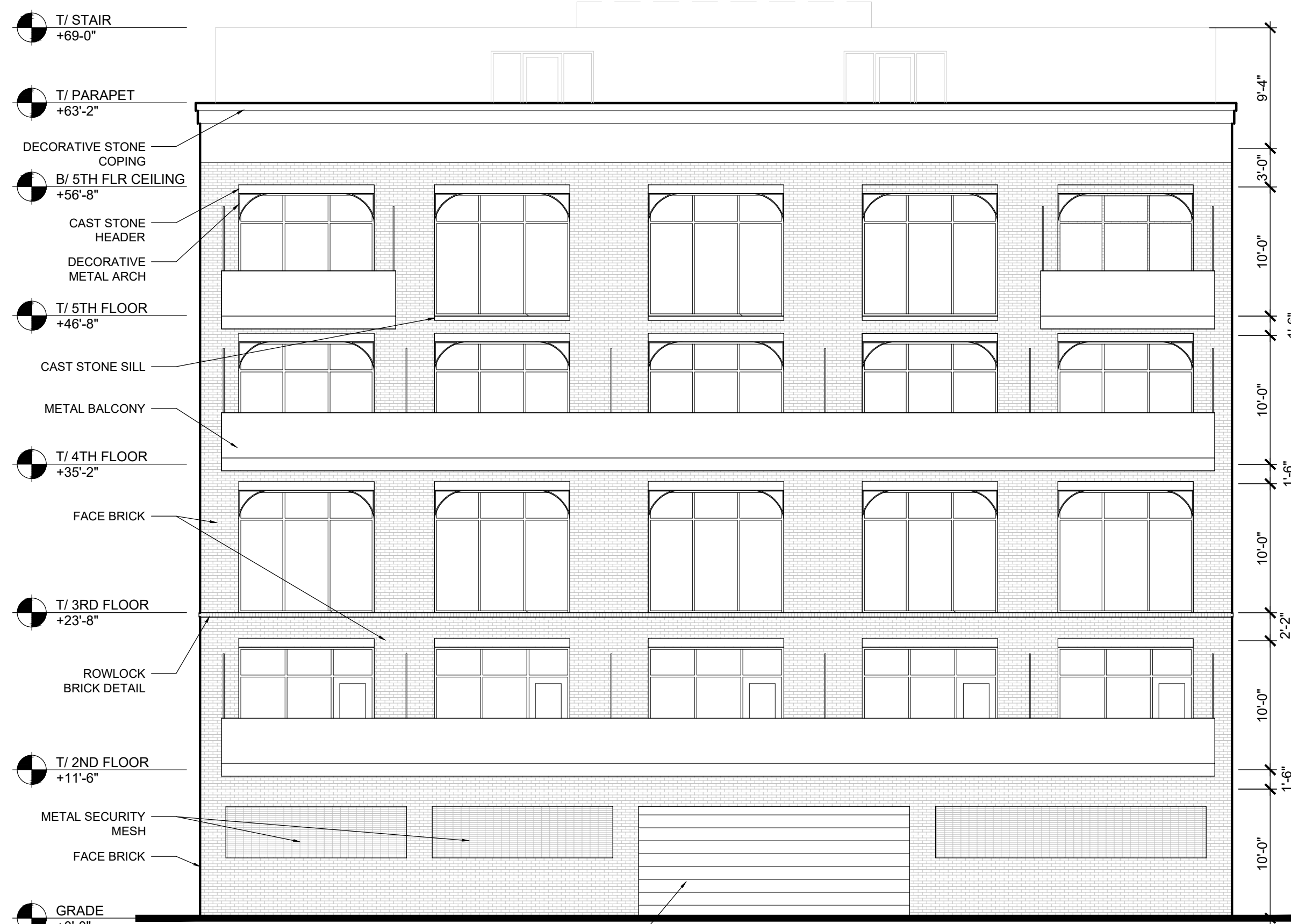
3 EAST ELEVATION SCALE: NTS
